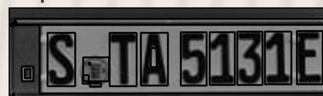
Step 7: Segment each character, apply bitwise_not mask for black and white, and apply small medium blur. Finally, pass it through Tesseract.
